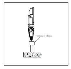
2). After the angle of light set, fasten the screw in the middle of adjustable arm. Make sure all connection is fine, then installation is done.r
