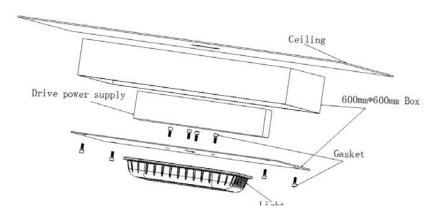
**Step 1:** Use 4pcs M8 screws to fix the fixture to the cover board of the Shoebox.
