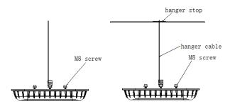
**Step 2:** Make the holes on the water-proof gasket go through the nuts of the M8 screws and put the gasket on the ceiling, then make the nuts of the M8 screws go through the keyholes on the mounting bracket, and turn the screws tightlyto fix the fixture to the mounting bracket.
