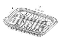
**Step 4:** Fix the LED driver to the driver box, and connect AC and DC wire, then fasten the fixed mount.
