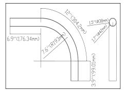
Installation pipe Mainly used for Dusk To Dawn Light 45W installation. Place the lamp on the mounting arm and lock it. Another side use of professional tools to drill two screw holes in the mounting bracket (wall or other).
