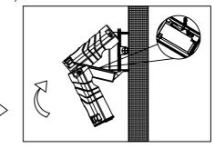
3 the upper cover and the lower cover are locked by screws (as shown).
