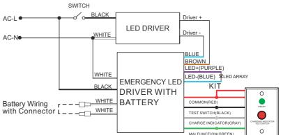
DO NOT MATE CONNECTOR UNTIL INSTALLATIONIS COMPLETE AND AC POWER IS SUPPLIED.
