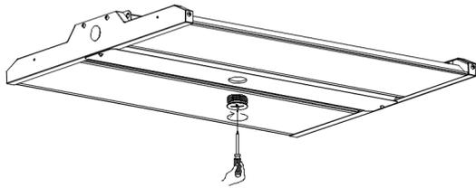
1. As shown in the picture, turn counterclockwise to unscrew the plug.
