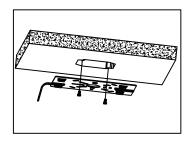
4.Slide the Canopy lights into bracket, and secure the screw on side of the light to prevent the light form sliding out from the bracket. Installation done.
