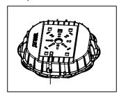
3.Attach the Canopy light with bracket by putting the ring on clips again. Connect the Black wire for line, white for Neutral, Yellow Green for Ground.
