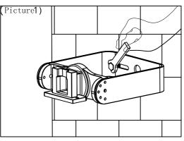
1. Fix the bracket on the wall and tighten the screw. (as shown in the picture)
