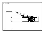
1 install the slip sleeve installer on the garden pole and tighten the screws, then connect the power cord. (as shown in the picture)
