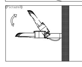
2. The luminaire is mounted on the bracket adapter, and tighten two fastening screws at the bottom of the bracket adapter, and then connect the power supply AC line of the arm adaptor according to the requirements. (as shown in the picture)
