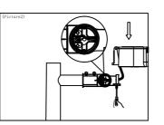
2. Fix the luminaire on SLIP FITTER and tighten the bottom screw. (as shown in the picture)
