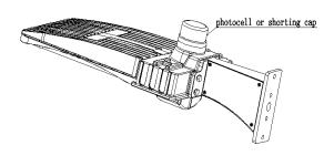
Replace shorting Cap with microwave sensor by Photocell with microwave sensor
