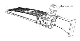
**Step 2** If it didn't work, open the waterproof box and set the microwave senor to work,lock the box after completed.(Attention put in the water-proof gasket before lock).
